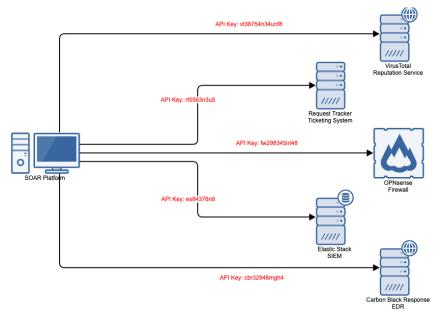
In IACD's API security experiments, a virtual enterprise was created containing multiple security products and services in the enterprise, controlled by a SOAR platform, with API keys managed by an API gateway:
