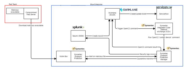
When the Symantec Endpoint Protection (SEP) anti-virus software on the Victim Box detects the malware download, the SEP alert is sent to Symantec Endpoint Protection Manager. The SEP Manager creates an alert in Splunk, which creates a record and initiates an automated workflow in the Swimlane SOAR product. The Swimlane orchestrator begins its workflow by creating a record and obtaining the relevant
